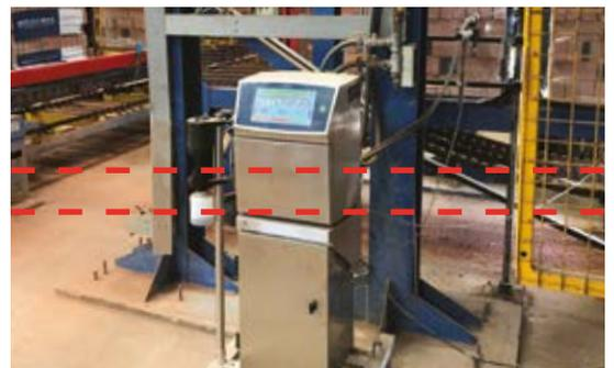
A UK based brick and concrete producer uses PrinterNet to remotely access their Linx 8900 printer located outside a safe area of their factory. The production line stops if the light beams in front of the printer are broken so being able to create and amend messages remotely is a perfect
